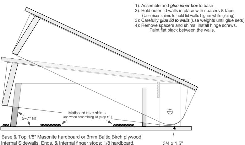
Internal Sidewalls, Ends, & Internal finger stops: 1/8 hardboard. External Lid Sidewalls & Ends: 1/4" Hardboard Glue all joints (use woodworking glue, no nails needed).
